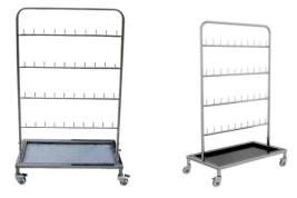
Stainless Steel Swab Stand with fifty spikes i.e five transverse bars with 10 spikes each complete with stainless steel drip tray at base mounted on four antistatic castor wheels, size 900\*500\*1600
