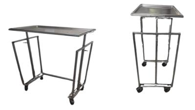
MAYO TROLLEY: overall size: 508 mm W X 826 mm L Adjustable from 814mm to 1340 mm. Bottom frame made of SS 304 tube of section 38X38 and 1.2 mm thick. Top frame of
